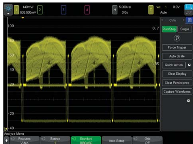
Figure 26: Triggering on 1080p HDTV signal analysis.
