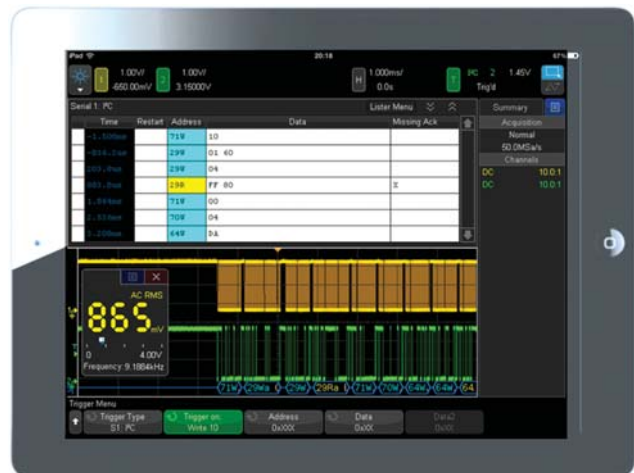
Figure 36: Tablet virtual front panel control.
