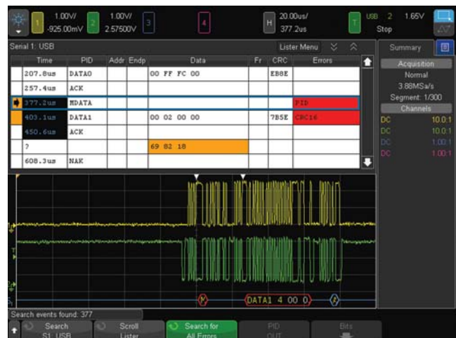
Figure 20: USB 2.0 trigger, decode and “lister” display.
