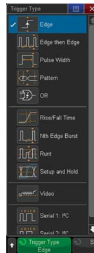
Figure 41: Wide array of advanced parametric trigger modes.
