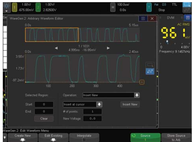
Figure 22: WaveGen arbitrary waveform editing screen.
