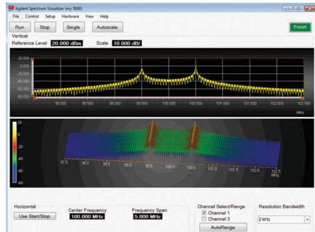
Figure 39: Waterfall view for ASV spectrogram measurements.
